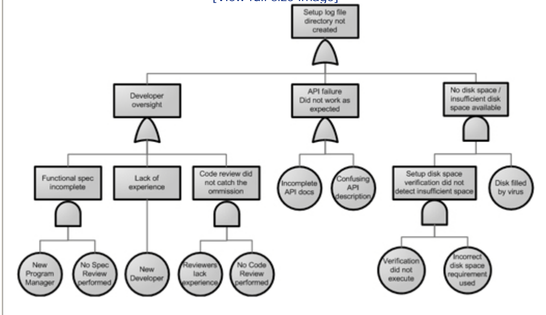
Figure 13-18. Complete setup logging fault tree for "Setup log directory not created"
