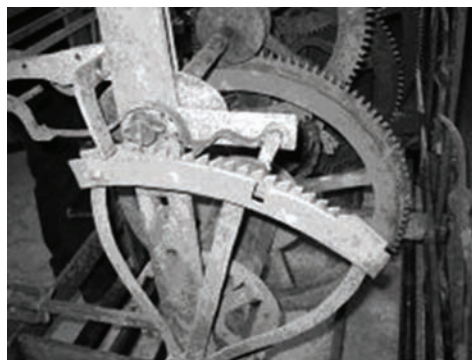
Figure 1. Organizations and machines: The internal rack and pinion mechanism of an 18 th century tower clock
